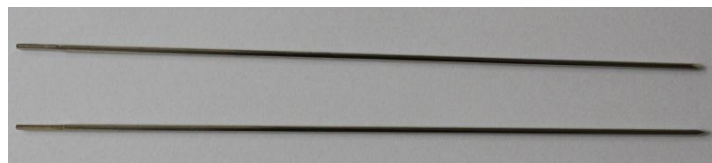
Figure 3.10: Guide pins (diameter – 3mm)
