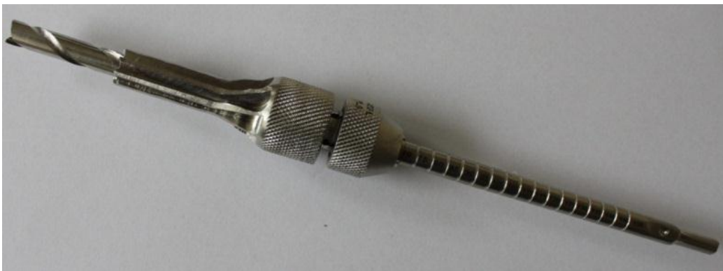
Figure 3.12: Generic triple reamer to make tunnel of three different diameters
