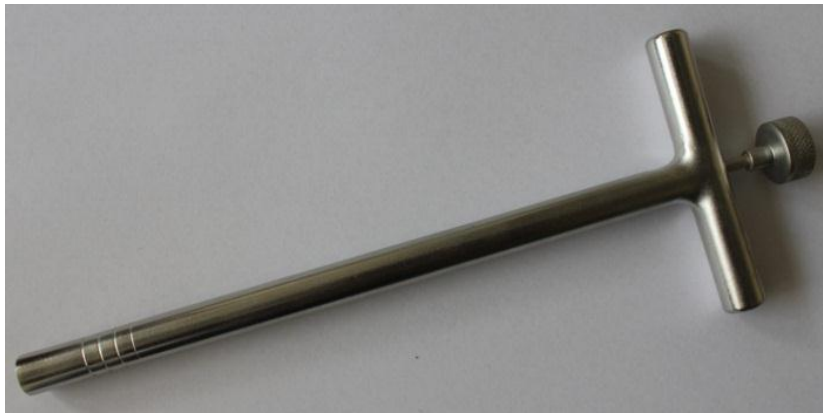
Figure 3.14: Generic insertion wrench
