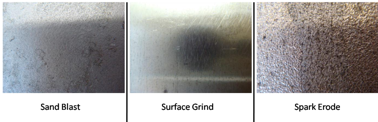
Figure 5.3: Surface finishes providing roughened texture on stainless steel samples
