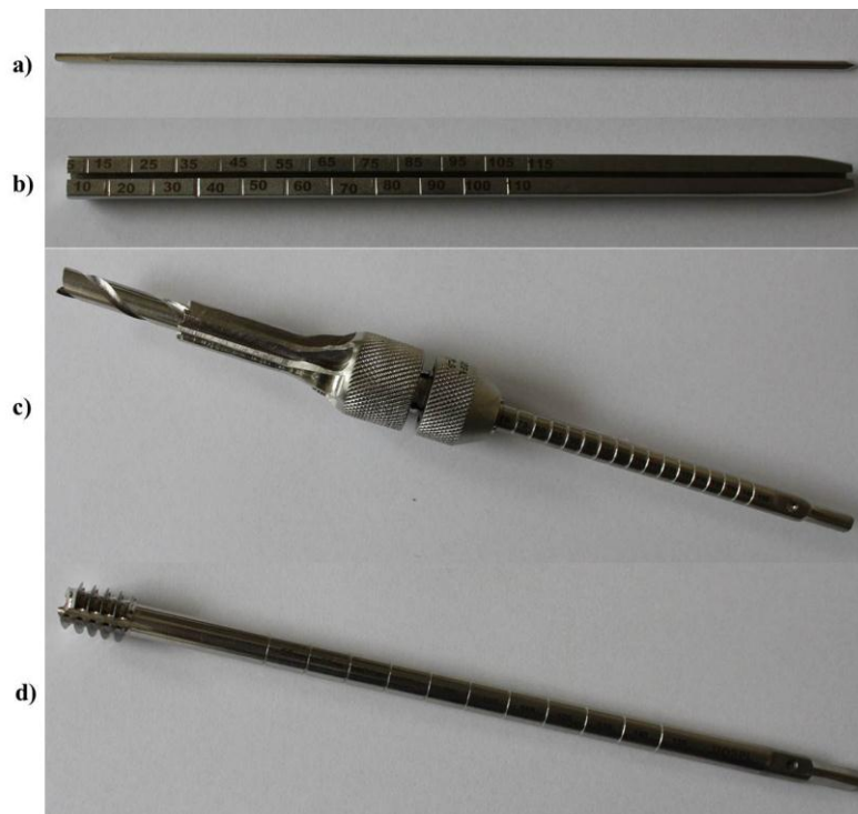
Figure 10.8: The other instruments to be used during the surgical procedure include: a) 2.5 mm guide pin, b) depth gauge, c) triple reamer, and d) tap. The instruments shown are manufactured by Sushrut Surgical Pvt. Ltd. (Pune, Maharashtra, India) for the generic DHS implant surgery.
