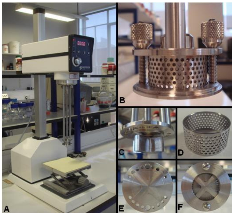
Figure 2.1 Image of the Silverson L5 M high shear laboratory mixer used in this work, showing: (A) mixer; (B) workhead; (C) rotor; (D) stator; (E) bottom view of the rotor; (F) bottom view of the work head. The workhead consists of a 4 bladed impeller (D: 31 mm, H: 12.5 mm) and an emulsor screen (D: 33 mm (ext.), H: 17 mm). A 0.175 mm gap is left between the edges of the rotor blades and internal wall of the stator (Silverson Machines Ltd., 2010).
