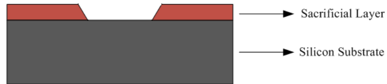
(b) Lithography and Development of the Sacrificial Layer
