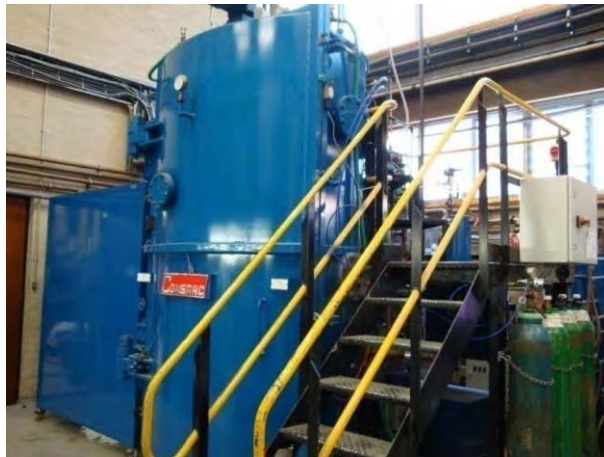
Figure 4 - 7. The vacuum chamber containing the Induction Skull Melting (ISM) furnace.
