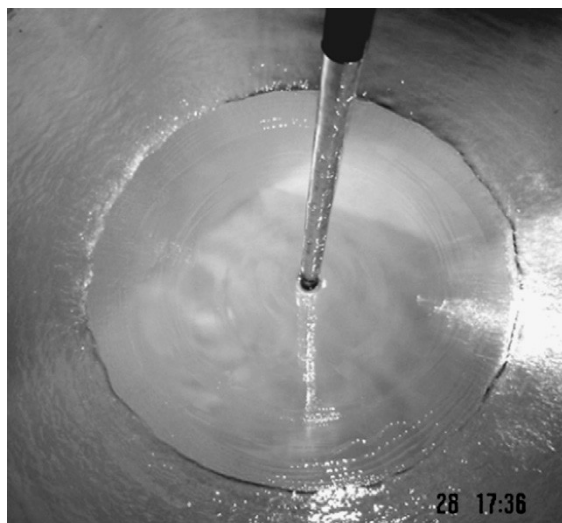
Figure 2 - 8. Circular hydraulic jump due to a normal impinging circular liquid jet (Kate et al., 2008).
