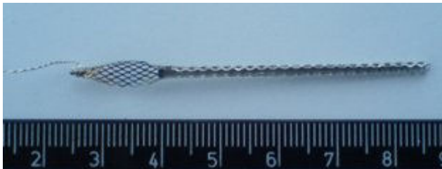
Figure 3.7 Showing the Ni mesh structure
