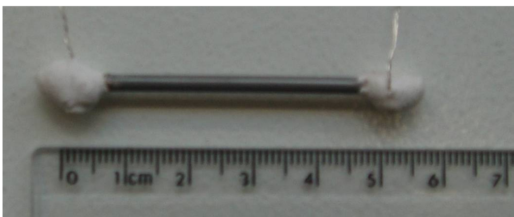
Figure 7.3. A tube prepared for electrical shock testing
