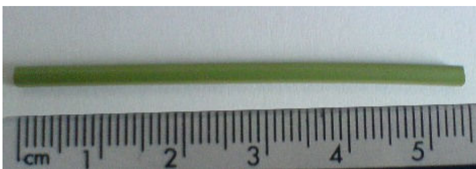
Figure 3.1 Image of the NiO/YSZ tube supplied by Adaptive Materials Inc
