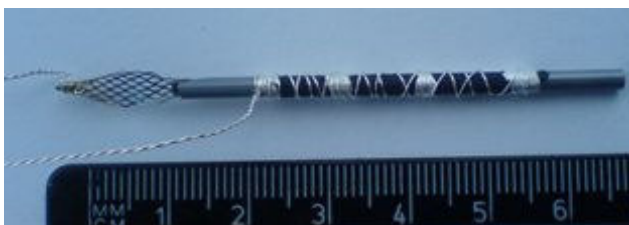
Figure 3.8. Showing a micro-tube with the Ni mesh inserted
