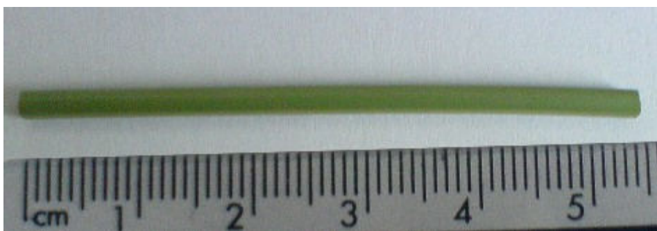
Figure 7.1. An anode supported micro-tube
