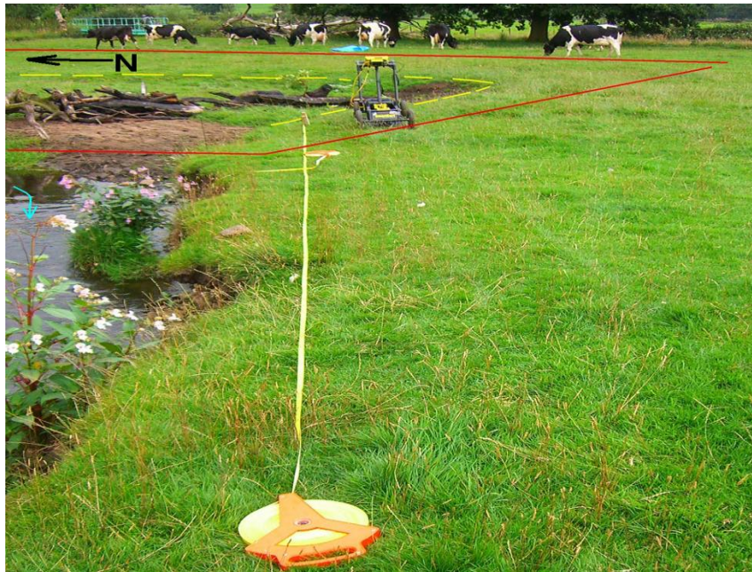
Fig. 4.1.11 Image of the Macclesfield site with the location of the ground-truth control GPR profile (presented in Figure 4.1.14), indicated by the tape measure, collected and correlated with the cut-bank of the River Dene (river flow direction indicated by blue arrow). Red line marks the location of the GPR grid and yellow line shows the edges of the recently filled eddy pool. Black arrow in the top left corner indicates the north (photo taken in August 2008).
