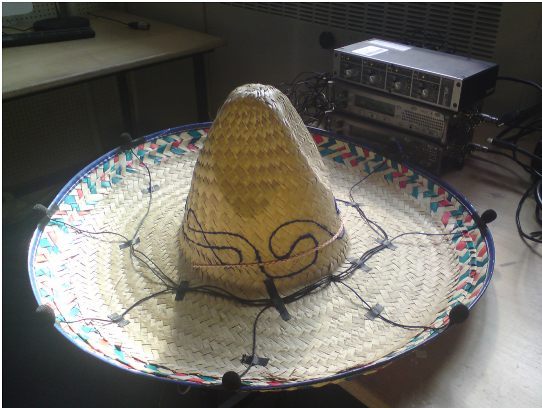
Figure 8. Sombrero mounted with 8 DPA 4060 and 4061 microphones connected to an RME Quadmic preamp and two SoundDevices 744T portable recorders.
