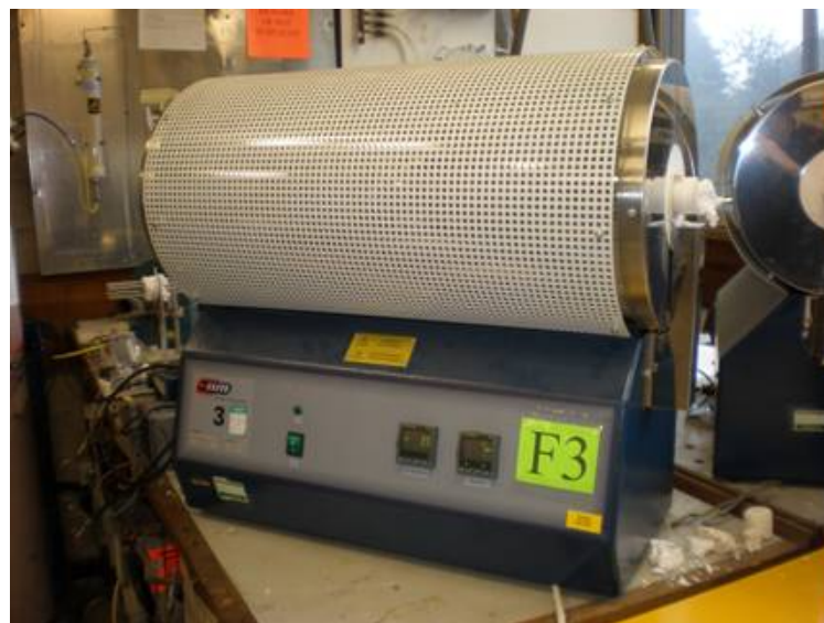
Figure 3.2. Photograph of the tube furnaces used for isothermal oxidation testing.
