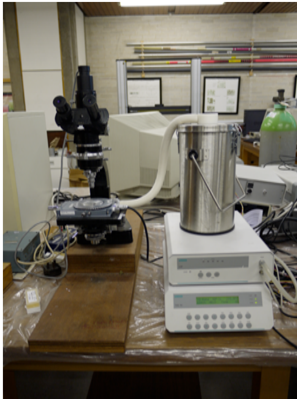
Fig. 4.11. Linkam TR600 hot-stage microscopy with controller.
