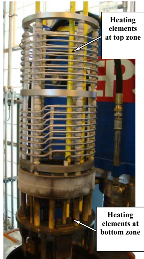
Fig. 3-4 The two zone molybdenum furnace used for HIPping.
