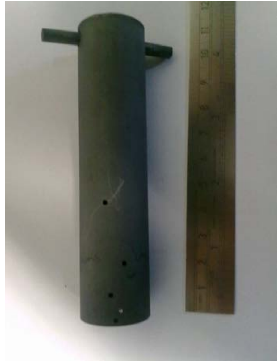
Fig. 3-6 Jominy bar with holes for holding thermocouples
