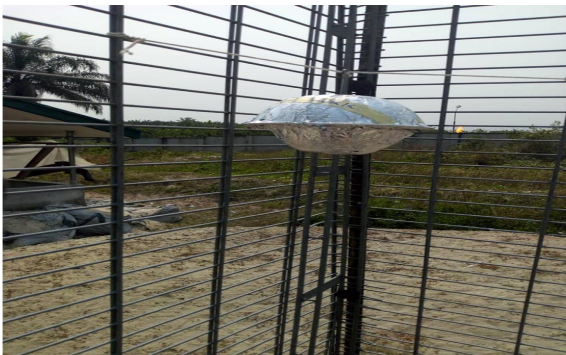
Figure 2-2 Passive air sampler deployed at a sampling location
