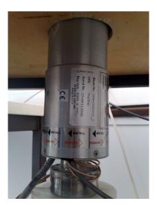
Figure 6.15: High Purity Germanium Detector
