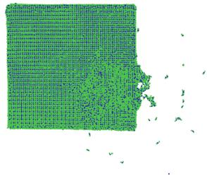
Figure 5.8: Sputtering of plutonium oxide (LAMMPS)[148]
