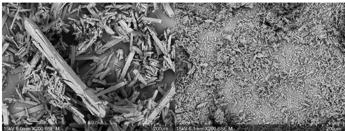
Figure 3.7) SEM images of HT-BIRM-1 (left) and RT-BIRM-1 (right) at 200× magnification
