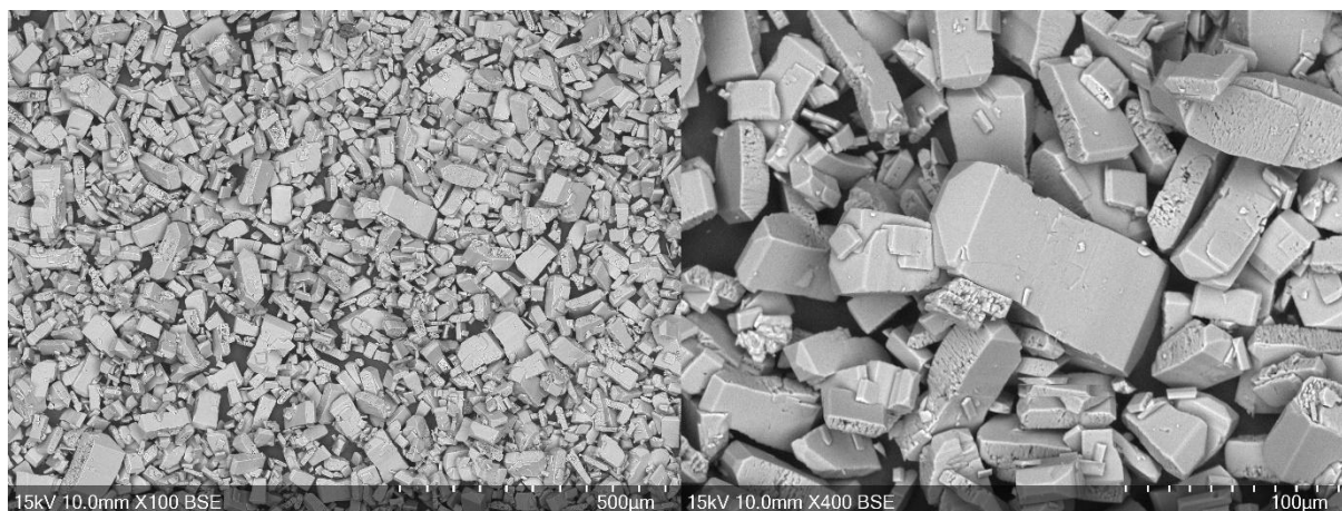
Figure 6.28) Two SEM images of BIRM-10 at 100 \times magnification (left) and 400 \times magnification (right)
