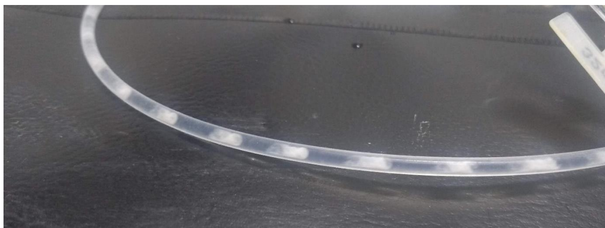
Figure 3.31) A section of tubing with just synthesised BIRM-1 flowing through; this tubing has an inner diameter of 1.5 mm.
