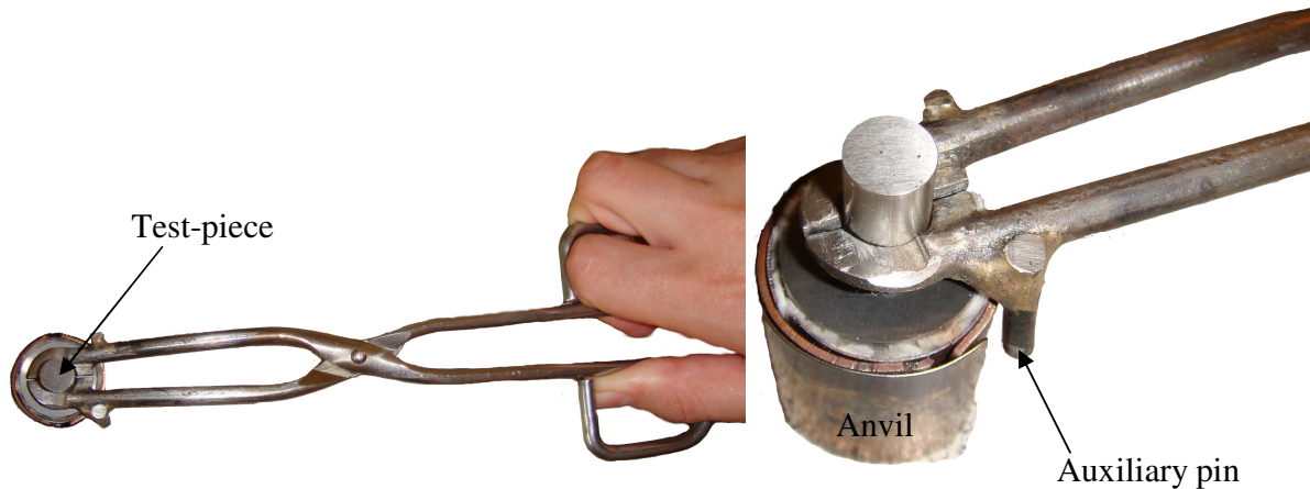
Figure 2.2 A tong was specially designed for placing the test-piece at the centre of the anvil.
