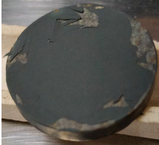
Figure 2.11: Spallated surface oxide on a Ti64 sample treated at 800 °C.
