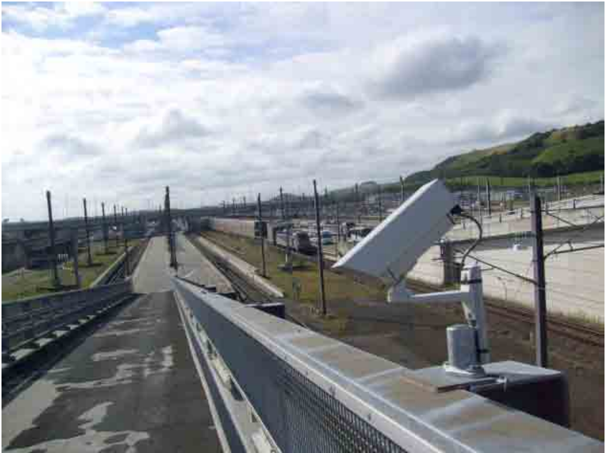
Figure 2.1 An IRIS remote infrared temperature sensor monitoring road surface temperatures at the Eurotunnel freight terminal in Folkestone, UK. Photograph courtesy of Campbell Scientific Ltd.
