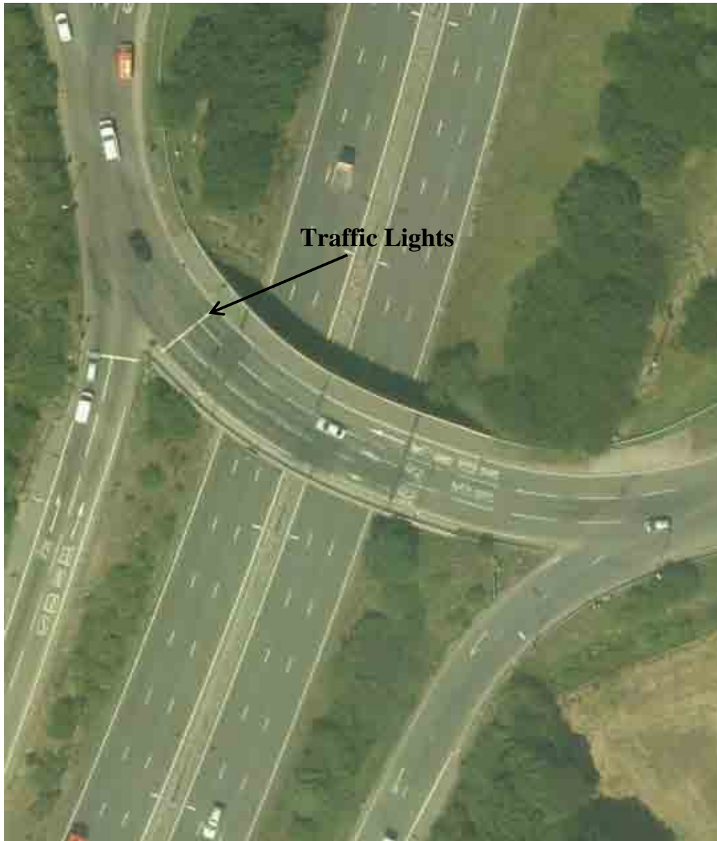
Figure 3.6 Aerial photograph of the motorway bridge identified in Figure 3.5(c), showing the location of traffic lights on the bridge which often leads to standing traffic causing the warm thermal singularity of +0.3^{\circ}\text{C} observed at this location.
