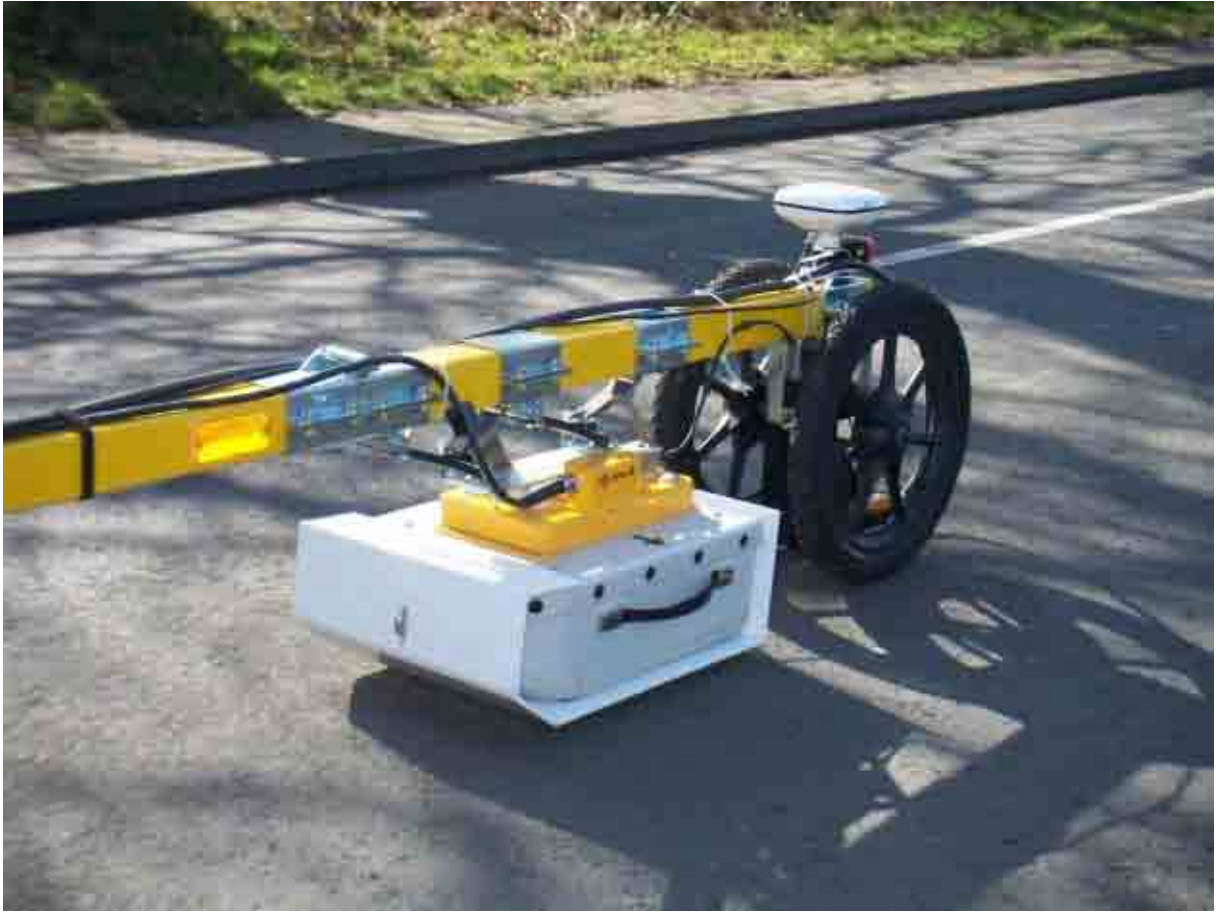
Figure 3.4 Equipment setup showing the Malå RoadCart in action.
