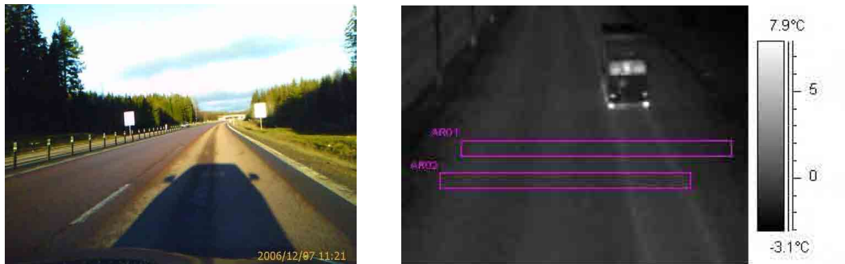
Figure 6.1 (a) Differential drying on the E4 highway north of Gävle, Sweden (approximately 60.5°N), showing how heat fluxes from traffic dry the road surface on the heavily trafficked inside lane, and (b) thermal image of the southbound M5 carriageway where frictional heat dissipation from tyre tracks is clearly evident (Chapman & Thornes 2008).
