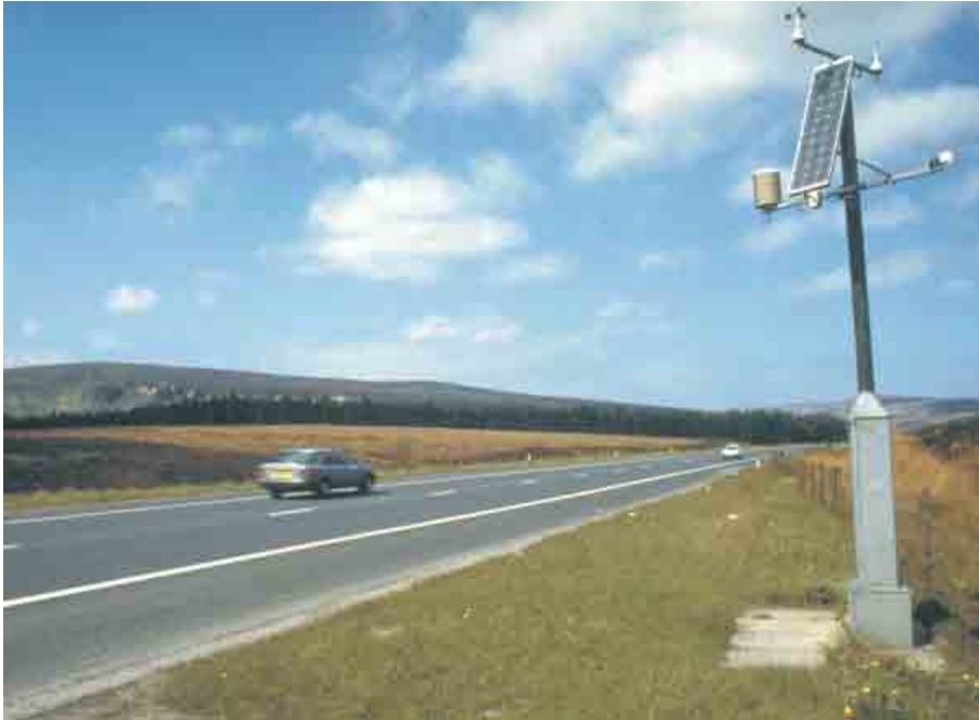
Figure 1.5 A Vaisala Road Surface Analyser (ROSA) outstation monitoring road surface and atmospheric conditions.
