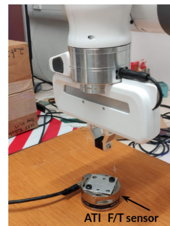
Fig. B.14 Task setup for comparing external FT sensor measurements with the robot's internal estimator.
