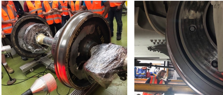
Figure 6.1 Wheelset defects search
