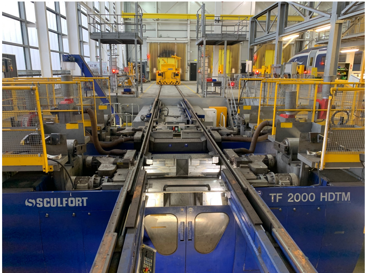
Figure 6.4 Wheel lathe in Temple Mills Depot
