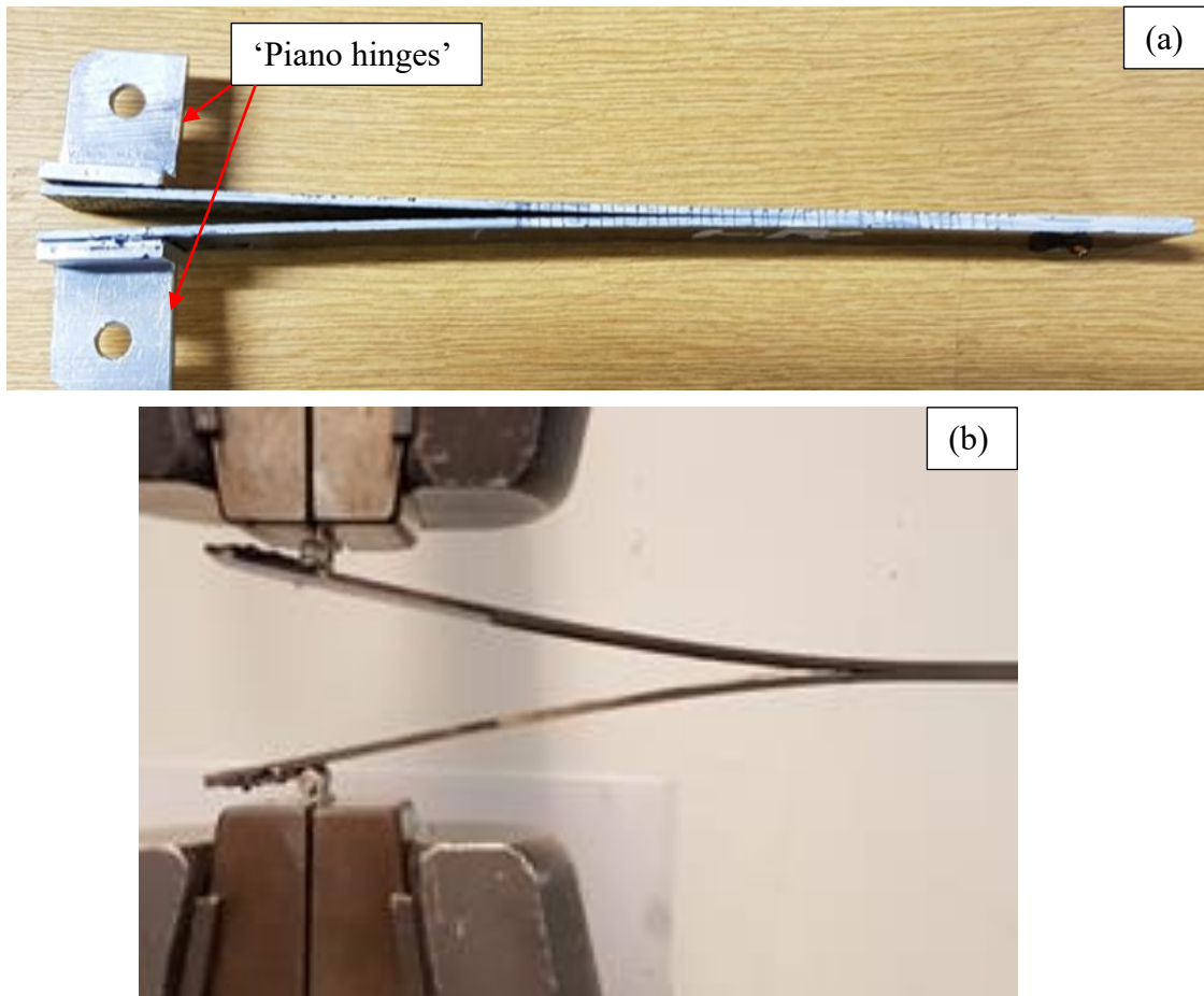
Figure 3.12 Images of (a) DCB specimen with piano hinges and (b) image of crack propagation during loading of Mode I interlaminar fracture toughness experiment.
