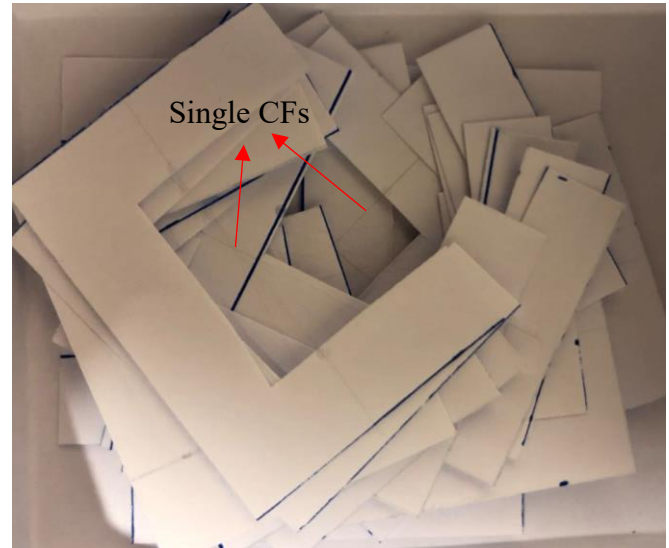
Figure 3.4 Paper frames with attached single fibre for tensile tests.
