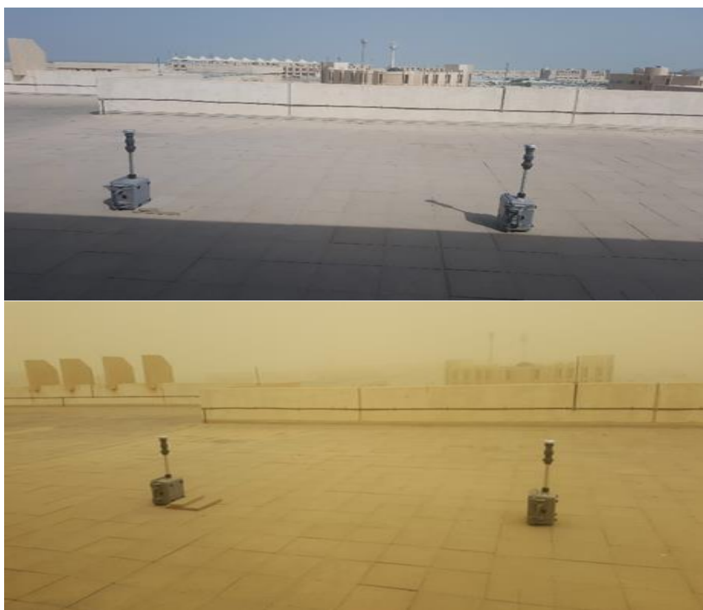
Figure 2.6 MiniVol samplers collecting samples at the University location during normal and dusty days.
