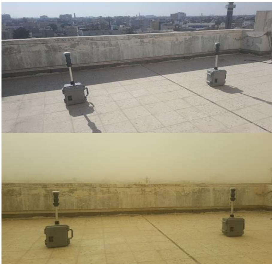
Figure 2.4 MiniVol samplers during winter campaign on the roof of Amanah during normal and dusty days
