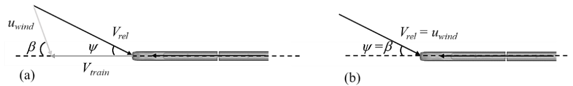
Figure 2.5: Vector diagram of wind and train velocities for (a) a moving train and (b) a stationary train, subjected to crosswinds.
