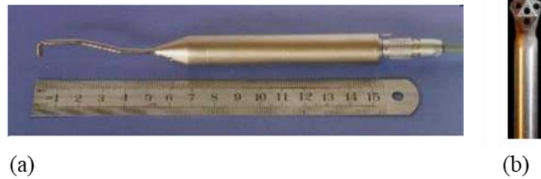
Figure 3.2: Series 100 Cobra probe (a) dimensional view (b) head view (Adapted from TFI, 2011).
