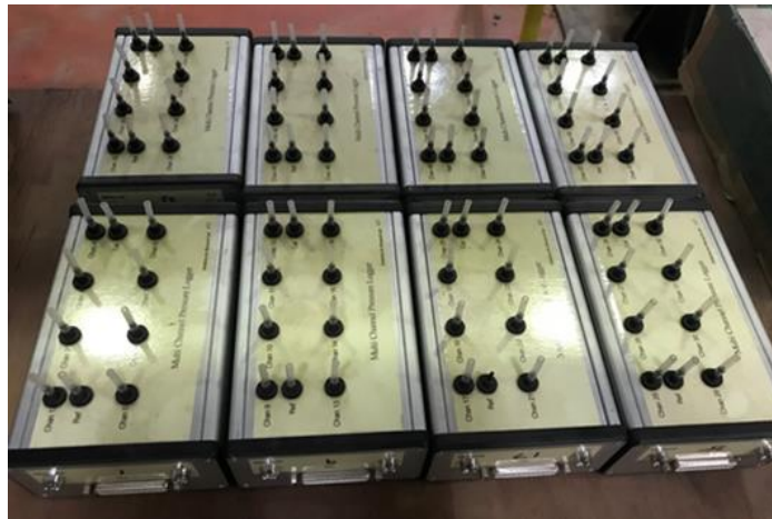
Figure 3.3: An image of the 8-channel modules of the Multi-Channel-Pressure-System used in this study.
