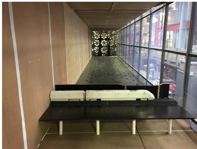
Figure 3.5: Setup of the splitter plate and other experimental models inside the wind tunnel at a yaw angle of 90^\circ .
