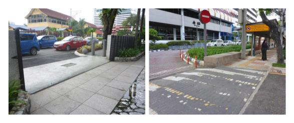
Figure 6-42 Examples of raised crossing to level with pavement
