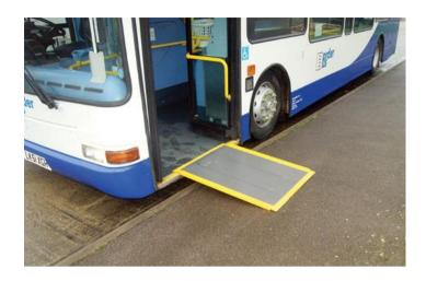
Figure 5-26 Ramp landed on bus stop get a gentle gradient
