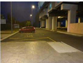
Figure 5-16 Drop-off and pick-up point in Alam Megah Station (a) high level of kerb without ramp or kerb cut (b) ramp provided near OKU parking but away from the pick-up point
