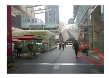
Figure 6-36 Accessible pedestrian walkway but inaccessible building entrance
