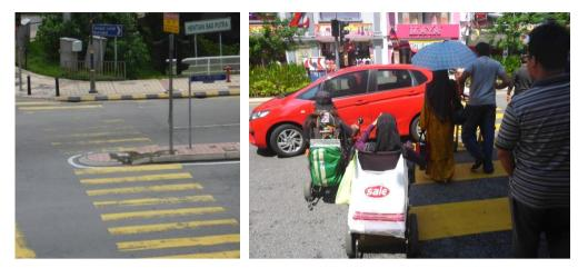
Figure 6-44 Examples of barriers in crossings (a) kerb as a barrier in the middle of the crossing (b) society's attitude that do not give priority for pedestrian to cross
