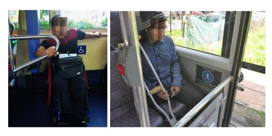
Figure 5-21 Facilities in an accessible bus (a) dedicated area to park wheelchair with a grab rail provided (b) priority seating for passengers with 'reduced mobility'
