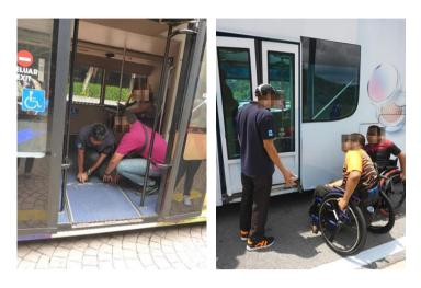
Figure 5-24 Maintenance issue in accessible buses (a) the driver trying to flip out the ramp using a lever (b) bus driver explaining the damaged door for wheelchair access to OKU passengers
