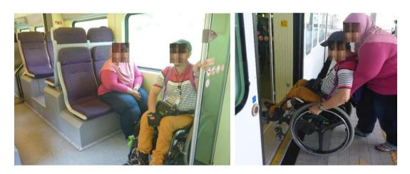
Figure 5-15 ERL experienced (a) coach without dedicated area for wheelchair (b) gap between the train door and the platform without the 'bridge'
