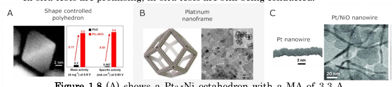
Figure 1.8 (A) shows a \text{Pt}_{2.5}\text{Ni} octahedron with a MA of 3.3 \text{ A mg}_{\text{PGM}}^{-1} . This image was adapted from Choi et al. 141 (B) shows a \text{Pt}_3\text{Ni} nanoframe with a MA of 5.7 \text{ A mg}_{\text{PGM}}^{-1} . This image was adapted from Chen et al. 144 (C) shows a Pt nanowire (left) and Pt nanowire with a NiO core (right) with a MA of 13.6 \text{ A mg}_{\text{PGM}}^{-1} . This image was adapted with permission from Li et al. 86
