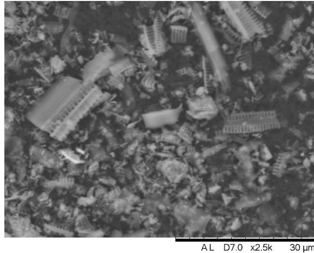
Figure 19 SEM image of diatomite particles
