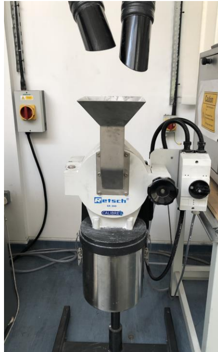
Figure 21 Shear mill used for grinding the PE granules
