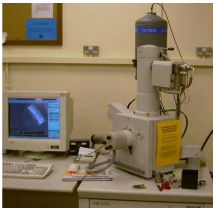
Figure 13: Image of the Philips XL30 EDX SEM used in sample compositional analysis. 39
