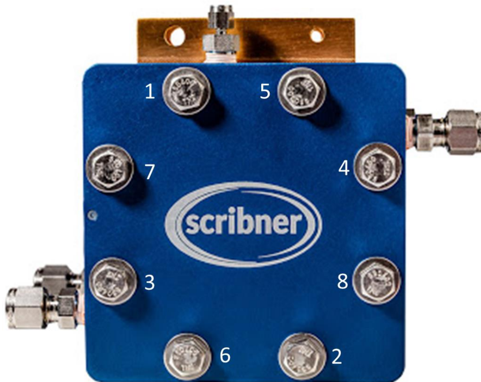
Figure 18 - Pattern in which bolts are tightened on the Scribner single cell test rig in order to ensure even pressure across the MEA held inside.
