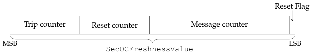
Figure 4.8: AUTOSAR freshness counter composition from trip, reset and message counters, and reset flag.
