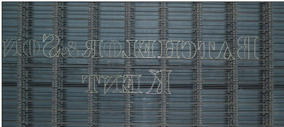
Plate 8. Example of a countermark sewn onto the surface of a papermaking mould © Simon Barcham Green, 2012.
