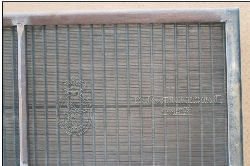
Plate 7. Example of a wire papermaking mould displaying a watermark and countermark. © Simon Barcham Green, 2012.
