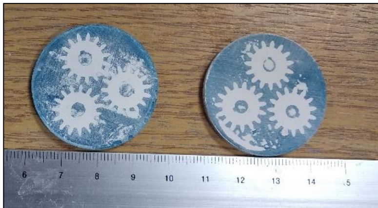
Fig. 4.30: Powder compacts within the moulds after ejection and gentle grinding
