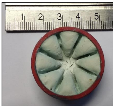
Fig. 4.22: Shrunken green body made from formulation 7, Walocel™ CRT as a binder
