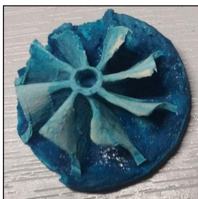
Fig. 4.23: Green body (approx. 35 mm dia) made from formulation 8, Aquazol® 500 as a binder
