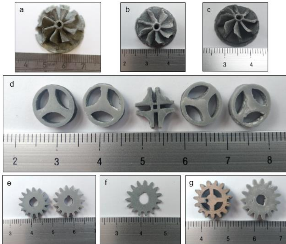
Fig. 4.33: Sintered Syalon 050 components (note: the scale in all the pictures is represented in mm), a, b and c turbocharger rotors fabricated in three different trials; d. circular sprocket gears and tools parts (four-sided) for welding; e. engineering gears (thickness >0.5 mm); f. engineering gear (thickness ~0.1 mm); g. flawed sintered components with visible pores and cracks
