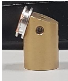
Figure 3.2: 70 degrees pre-tilt EBSD holder
