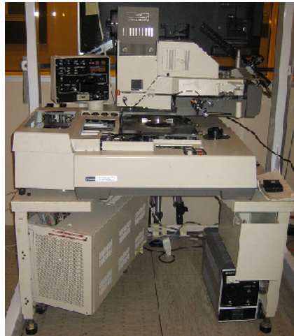
Figure 6.8 Mask aligner machine (PLA-501 FN) for photolithography process
