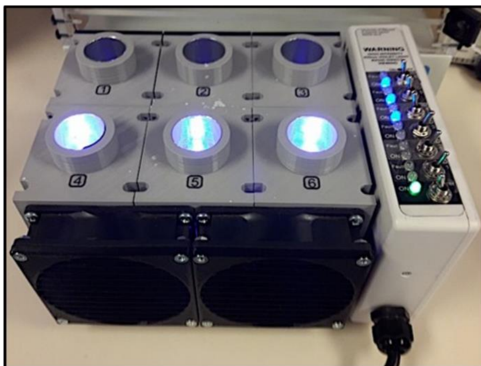
Figure 6.11: Photo of photoreactor set-up used for photoinitiated polymerizations in this chapter.
