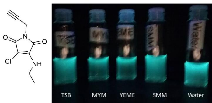
Figure 5.5: Structure and photo of fluorescence under UV illumination of ACM 5.8 after 24 hour incubation in cell media.
