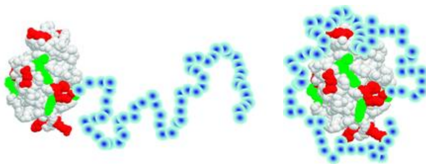
Figure 2.4: Topology of enzyme conjugated PEG (left) versus the incorrect, commonly assumed 'shroud' model (right). Figure reproduced from Pai et al. 44
