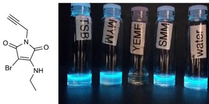
Figure 5.4: Structure and photo of fluorescence under UV illumination of ACM 5.4 after 24 hour incubation in cell media, showing YEME quenching.
