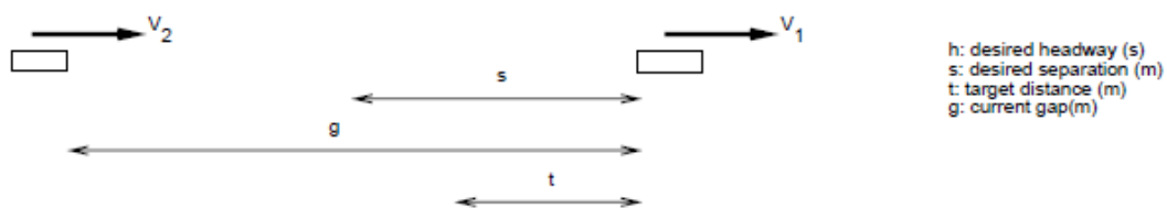
Figure 2.1: Diagrammatic overview of the relationship between the lead and following vehicle (Duncan, 1998)
