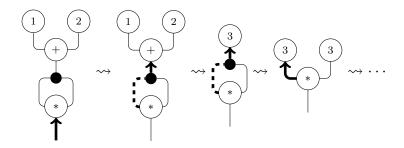
When the token passes through the contraction •, it remembers its old position, as indicated by a dashed line. This record is necessary to determine a token position after the duplication. In the rewrites-first DGoIM, the record of previous positions is the only part of the token data that depends on underlying graphs, namely a box stack (see Def. 2.3.1).
