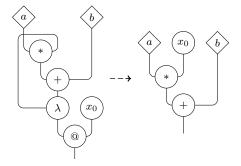
Observation of the resulting network, which involves parameter nodes, can be achieved solely by token passing. The output data  $a * x_0 + b$  can be obtained by letting the token travel through the network from the bottom, as indicated by a thick gray arrow:
