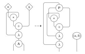
Graph abstraction is not a local rewriting rule, because it extracts *all* parameters in a network, which are not necessarily neighbours of the triggering node 'A'. Parameters are extracted altogether as a function argument, so that parameter update can be completed with graphical beta reduction. This deviates from the in-place update of TensorFlow. Once a new parameter vector (a', b') is computed, pre-
