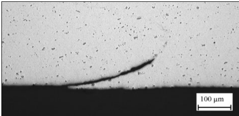
Fig. 2. 31 Characteristic root flaw in FSW 2014A caused by using a too short pin in 5083 alloy[109]
