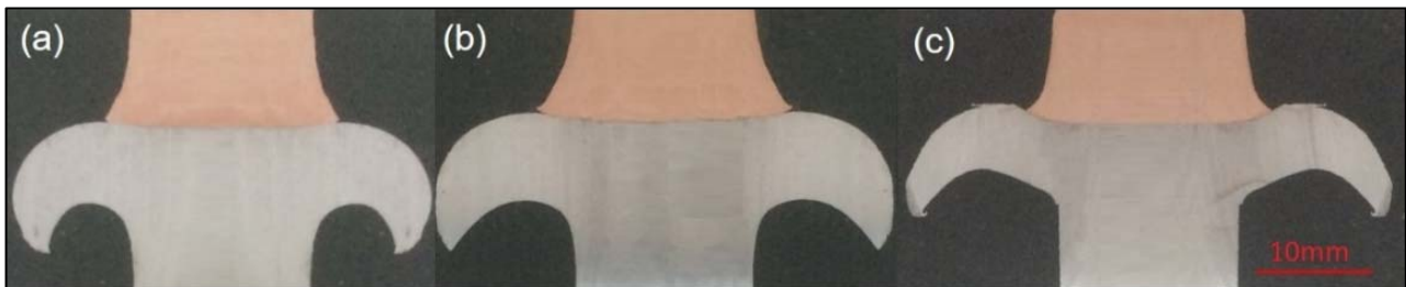
Fig. 6. 10 Flash formation at the Al weld side (bottom) of LFW joints welded under different forging pressures. (a) 110MPa, (b) 80MPa, and (c) 60MPa
