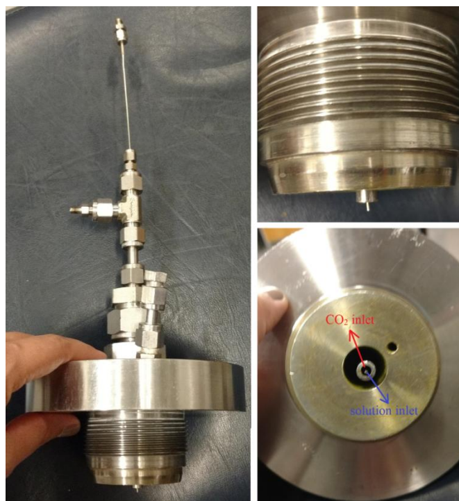
Figure II-2. Lid of high-pressure vessel (500 ml) with detail of solution and CO 2 injection for SAS.
