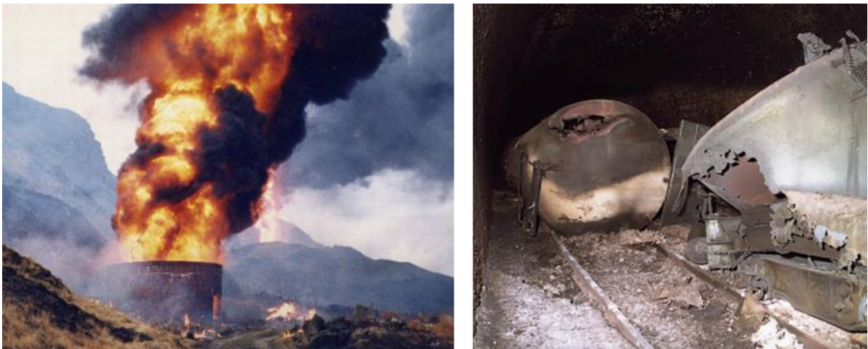
Figure 7: The Summit Tunnel accident and subsequent fire caused by the derailment of a train carrying fuel. The derailment was initiated by a faulty axle bearing that led to the rupture of the axle while the train was moving through the tunnel derailing the train [28].
