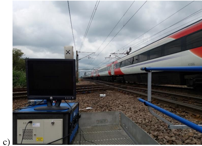
Figure 100: a) Photograph of the Newark flat crossing, b) the installation process of the AE system overnight and c) measurement setup and example rolling stock moving over the crossing at normal operational speed.
