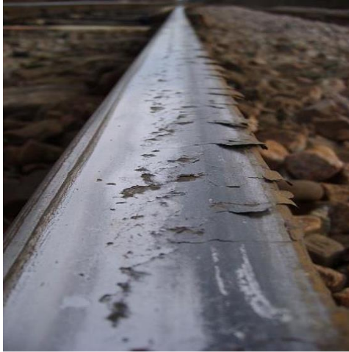
Figure 18: RCF cracks with high level of plastic flow (photo courtesy of Brian Whitney, Network Rail)
