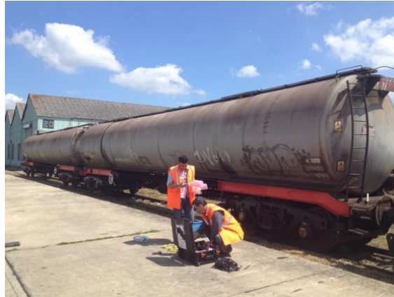
Figure 41: Tanker freight wagons with several axel bearings artificially damaged in the roller or race using a power tool.
