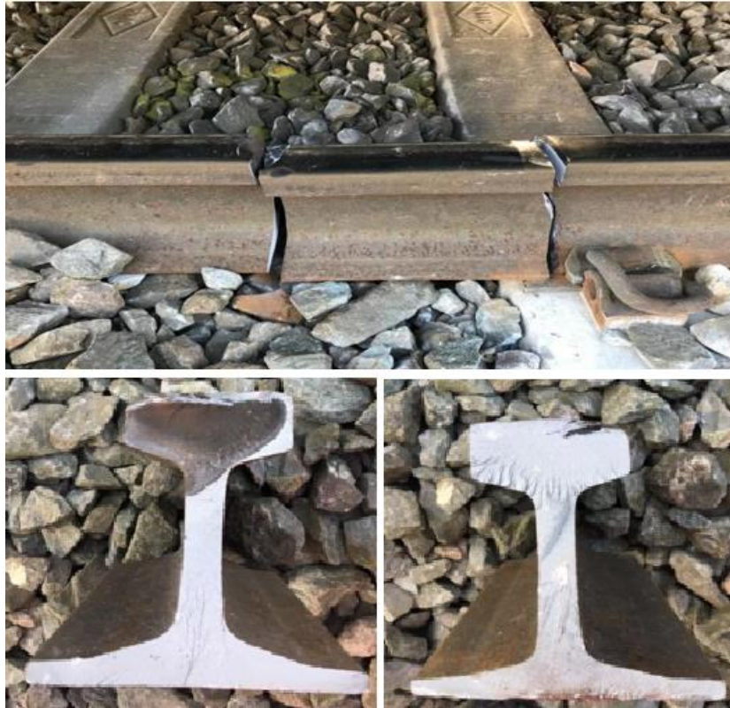
Figure 21: Photograph showing classic fatigue crack (courtesy of Brian Whitney, Network Rail)
