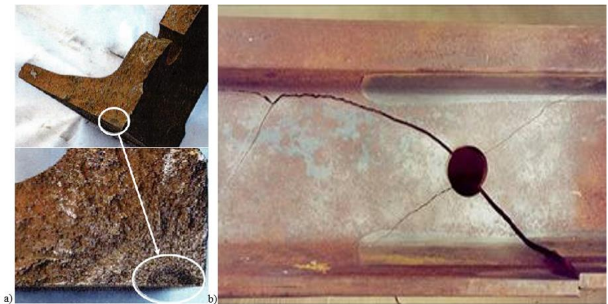
Figure 22: a) Rail foot corrosion (courtesy of Brian Whitney, Network Rail) and b) bolt hole cracking [53].
