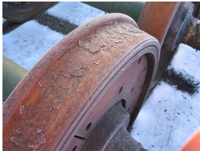
Figure 12: Metal build-up on the surface of the tread of a freight monoblock wheel.
