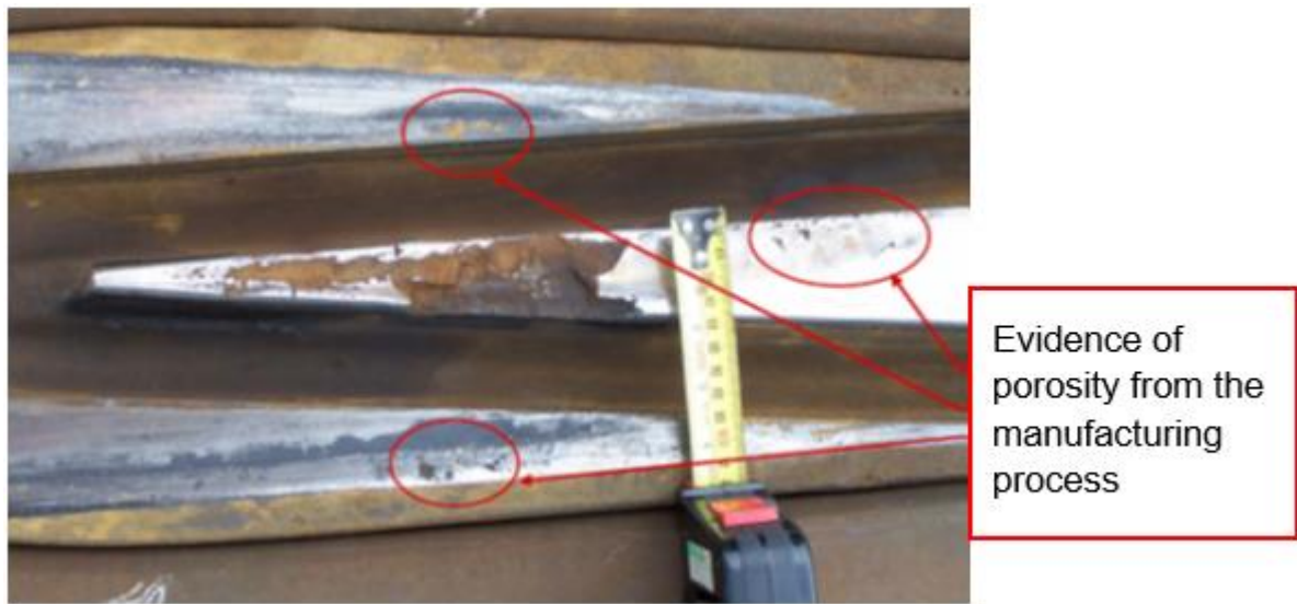
Figure 26: Photograph of damaged crossing showing evidence of porosity due to the manufacturing process (the photograph is from Hardface Technology Presentation on Repair and Rebuild of Manganese crossings using Hardface Welding, 2003).
