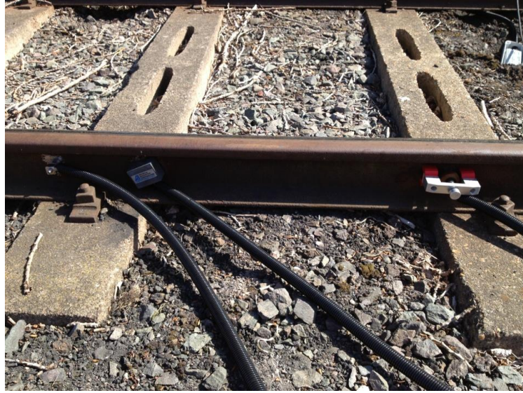
Figure 44: Wayside installation of AE sensors and accelerometers at Long Marston.
