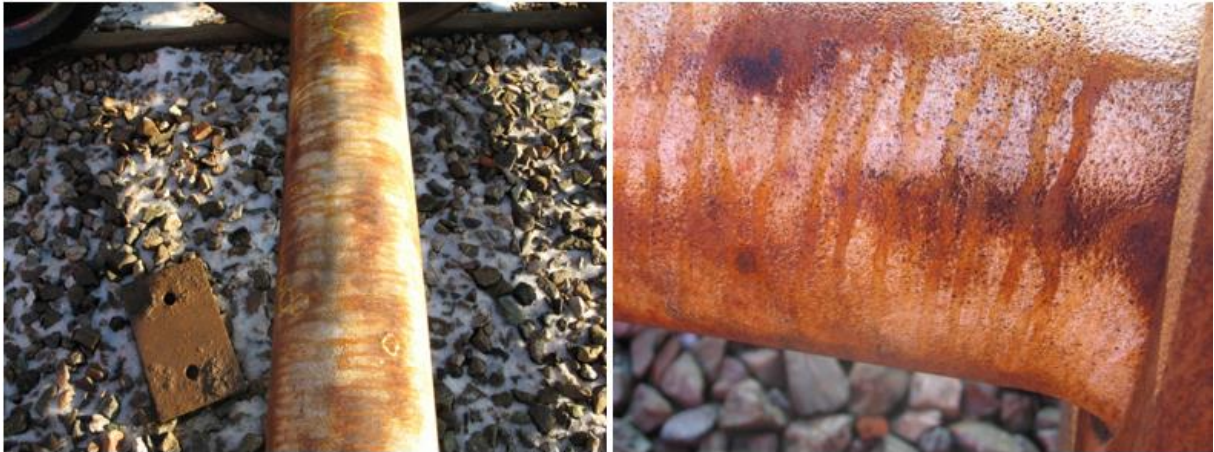
Figure 17: Photographs of pitting corrosion on a freight axle.
