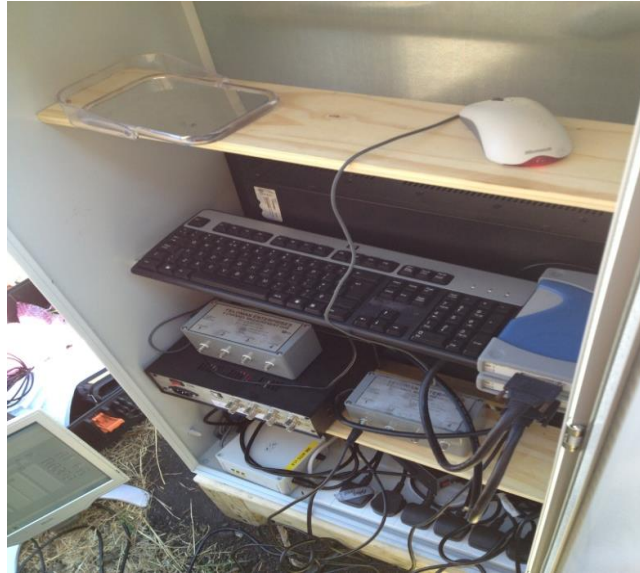
Figure 42: The customised data acquisition equipment used during trials at Long Marston.
