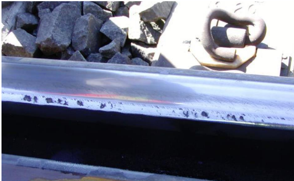
Figure 19: Shelling of the running surface of the rail [53].
