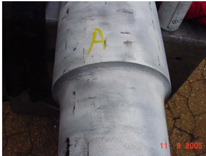
Figure 16: Photograph of fatigue cracks on the surface of the axle (Courtesy of Dr John Rudlin, TWI Limited).
