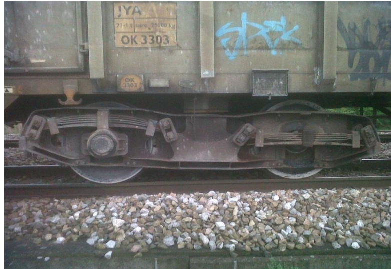
Figure 15: Photograph showing a sheared axle bearing (Courtesy of Mr. Nick Pinder, Network Rail).
