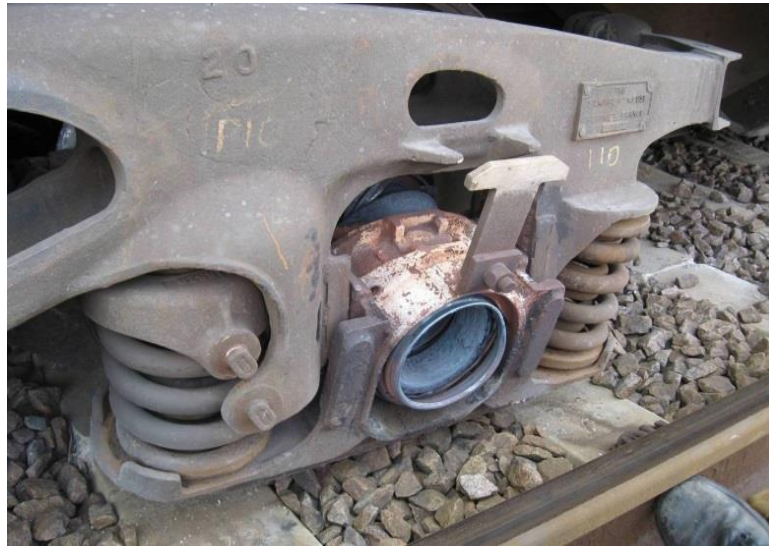
Figure 14: Derailment due to axle bearing failure (courtesy of Mr. Nick Pinder, Network Rail).
