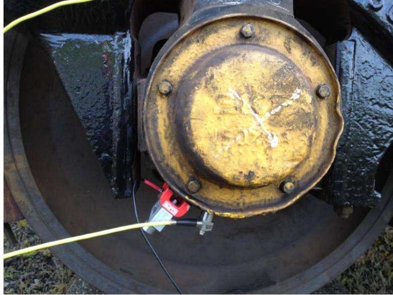
Figure 43: AE sensors and accelerometer installed in one of the axle bearings of the tanker freight wagons tested in Long Marston.
