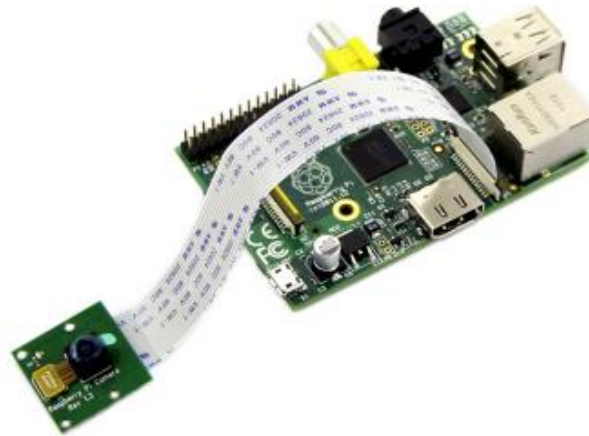
Figure 2.8 – Raspberry Pi computer board with attached Raspberry Pi camera module ( Nguyen et al., 2015 ).
