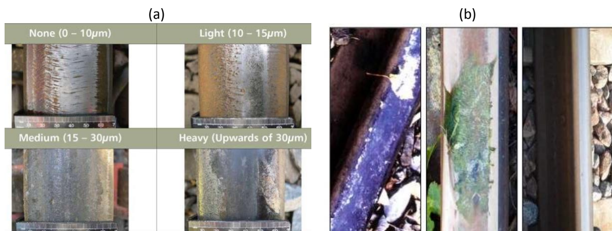
Figure 1.8 - (a) Adhesion coefficient recorded on a rail track, (b) Visual leaf contamination along the rail network ( Adhesion Working Group, 2018 ).
