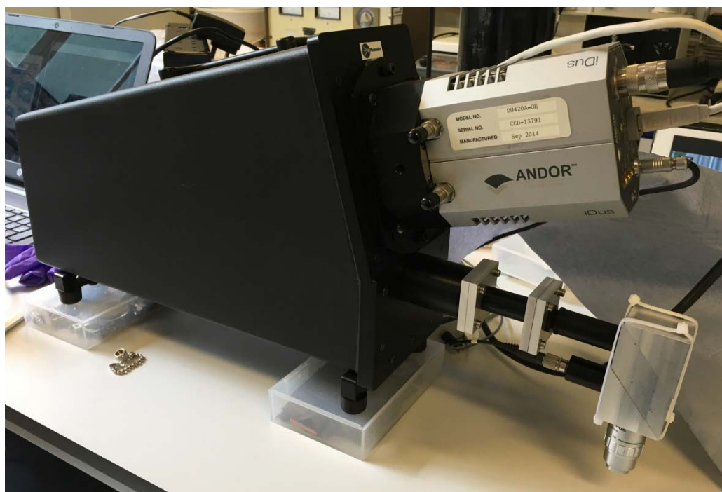
Figure 5.13: Photograph of the overall Raman setup. The echelle spectrometer is on the left hand side with the Raman collection setup machined from aluminium on the right hand side. The Andor cooled CCD is visible in the top right hand corner.
