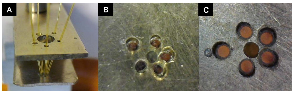
Figure 5.10: Photographs of (A) the fibre optic arrangement with a top bar supporting the fibres coming in and allowing the laser beam through without any fibres getting in the way; (B) the fibres coming through the 300 \mu m holes in the exit bar and also demonstrating the damaging of the outer covering of the fibres by the sharp edges of the holes and (C) the polished fibres where the five collection holes are not perfect in distance from the centre laser hole, resulting in a non-consistent collection angle.
