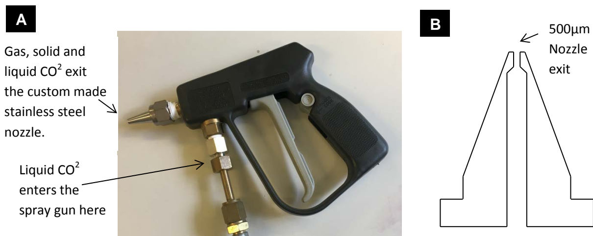
Figure 2.3: (A) Photograph of the spray gun converted with PTFE washers inside and a custom exit nozzle used in the CO 2 snow cleaning system. (B) Schematic cross section of custom nozzle.
