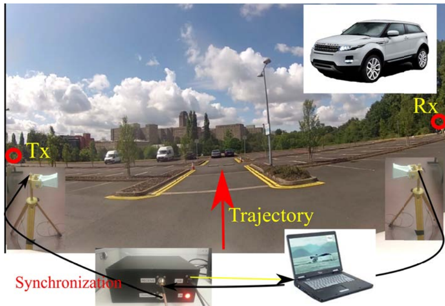
Figure 6.9: Target's point of view of the experimental set-up.
