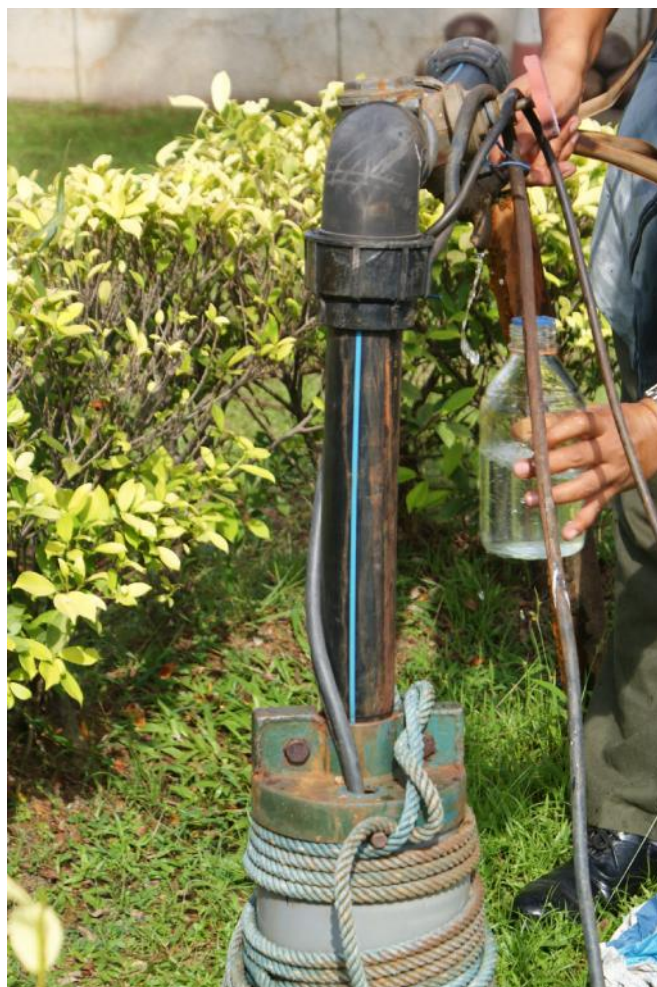
Figure 6.1 Water sample is taken directly from the well through sampling tap.
