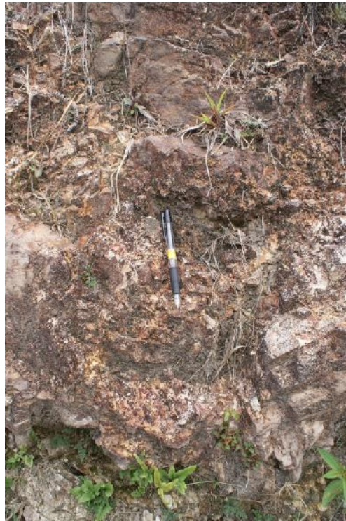
Figure 3.16 Iron oxide-hard crust in a fault zone in Shah Alam.
