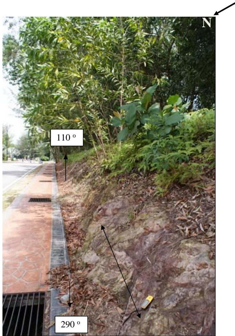
Figure 2.42 b) The wider joint spacing in massive quartzite at outcrop B (Location 2).
