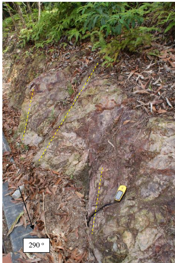
Figure 2.41 Joint in quartzite ranges from 0.5 to 1 metres length. The size of the GPS device is 10cm. The yellow dashed lines are the main joint set observed at Location 1
