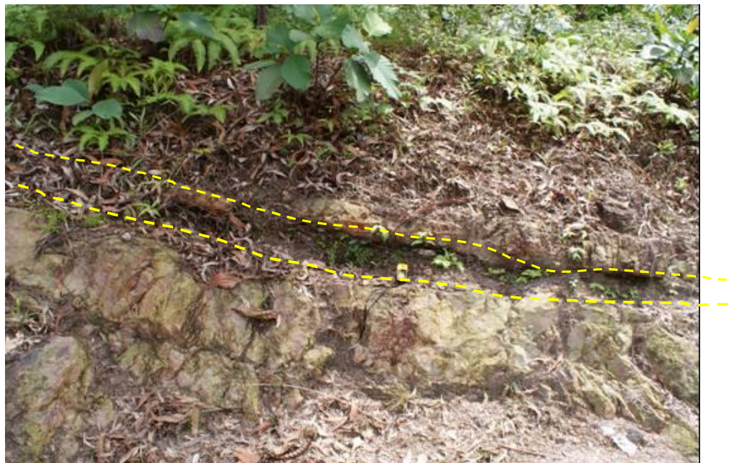
Figure 2.26 The sandstone with thin bed of shale (between yellow lines) at Outcrop B. The rock sequence is dipping to the southwest at an angle of 12^\circ . The GPS device is 10 cm in length.
