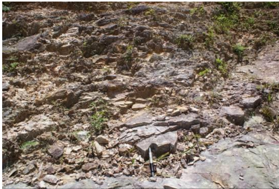
Figure 2.47 The joint sets in the hard grey shale at Outcrop C.
