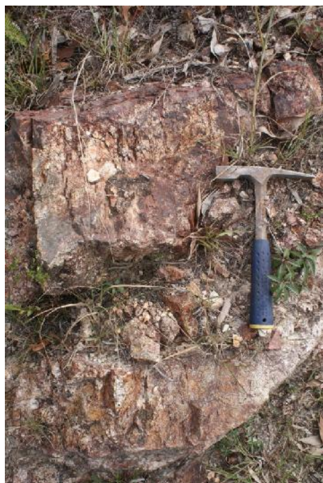
Figure 3.22 Bedding planes and joints in sandstone heavily coated with iron oxide in Shah Alam
