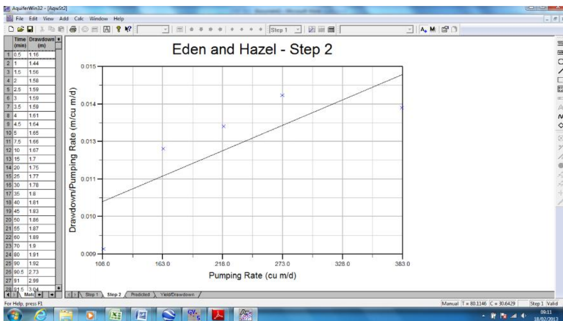
Figure 5.20 An example of well where the Eden & Hazel method was attempted (Mitsui High Tech)
