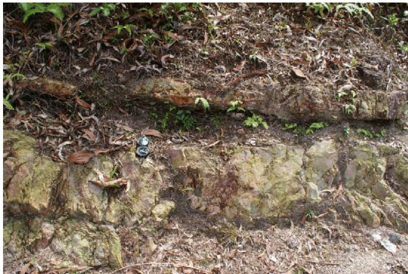
Figure 3.13 Bedding plane joints in Shah Alam, possibly developed somewhat due to weathering in shale layer
