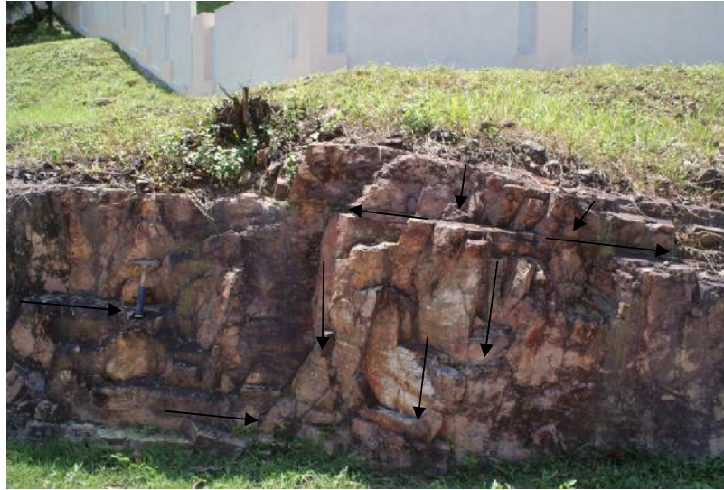
Figure 3.12 Water movement in quartzite in Shah Alam. In this case, water is assumed to flow along approximately vertical joints that are perpendicular to the bedding and then along the approximately horizontal bedding plane joints.
