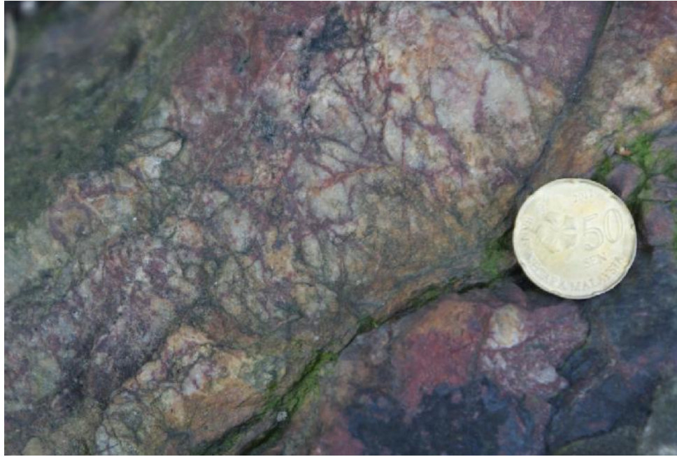
Figure 2.36 Fine fractures in mottled sandstone. The fractures are filled with iron oxide. The diameter of the coin is 2.3cm.
