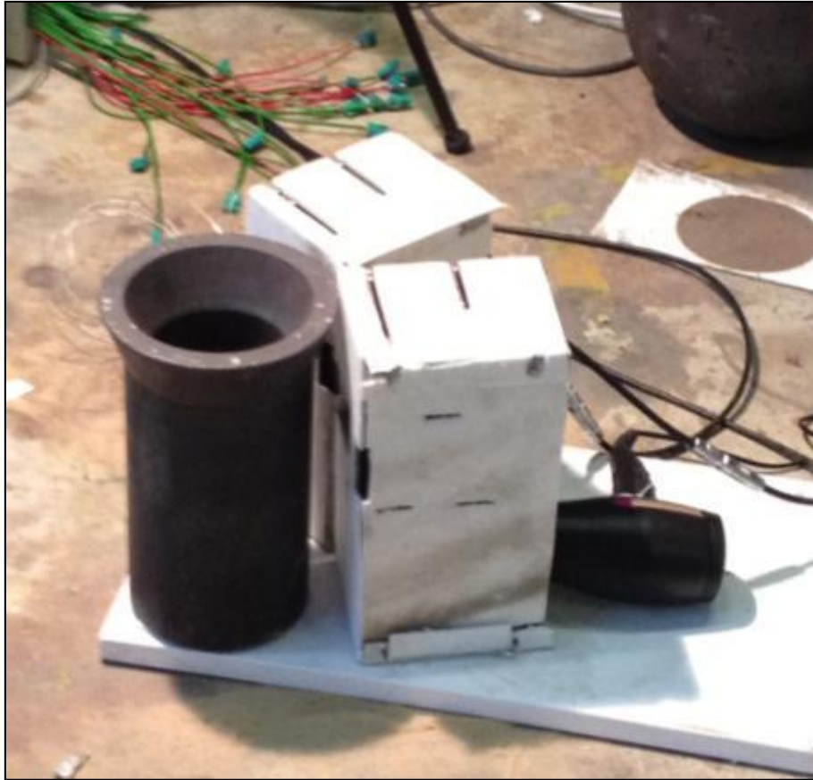
Figure 4-4 – Photograph of the air-gap experimental set-up displaying the mould and housings for the laser triangulation sensors sitting on top of the slab of fireclay.
