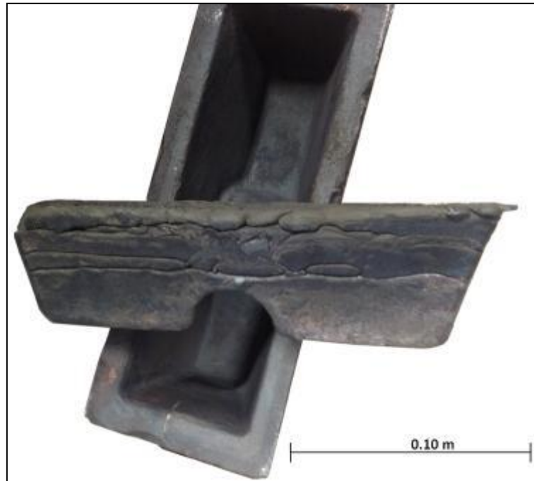
Figure A-2 – Photograph of an as-cast billet containing entrained oxide surfaces (i.e. laps)
