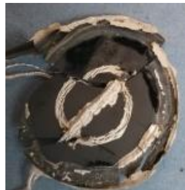
(f) SOFC-10D-2, post-150 hours on biogas
