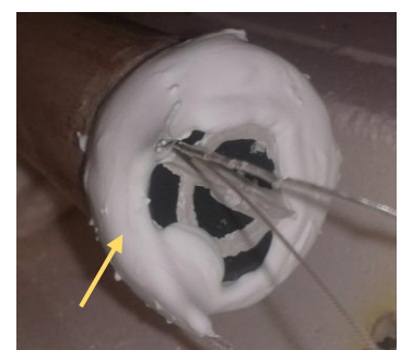
(c) Ceramabond excessive seal expansion
