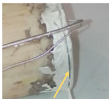
(a) Thin Ag seal delaminated
