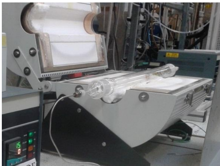
Figure 6.1: The rig configuration used for dry reforming of simulated biogas
