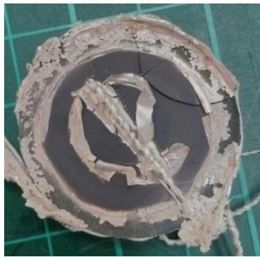
(c) SOFC-4D-2, post-22 hours on biogas
