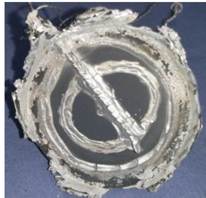
(b) SOFC-2D-1, post-22 hours on biogas
