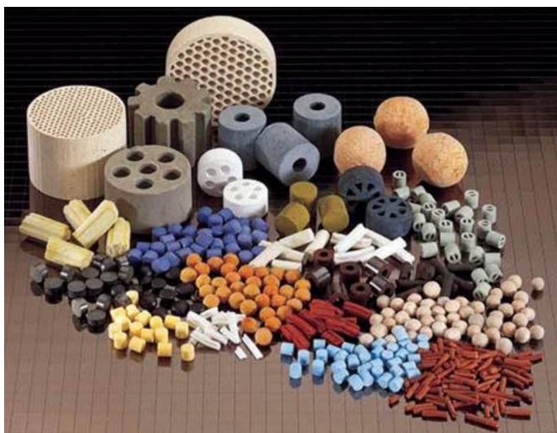
Figure 2.2. Commercial heterogeneous solid catalysts with different shape and structure for refineries and petrochemical applications (Süd-Chemie, 2014).
