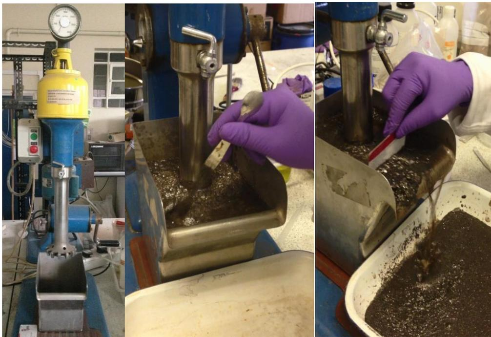
**Figure 4.5: Left to Right - A Denver flotation cell; 2 minute froth conditioning; 3 minutes scraping**
