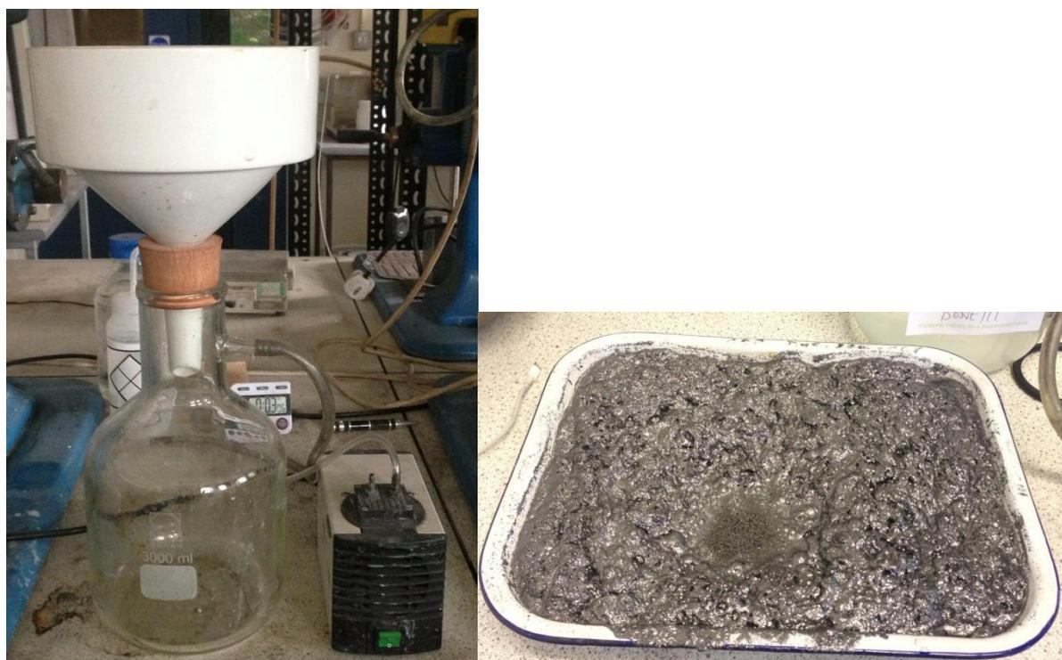
**Figure 4.6: Left - Vacuum Filtration Unit; Right - Graphite Froth in collection tray before filtration**
