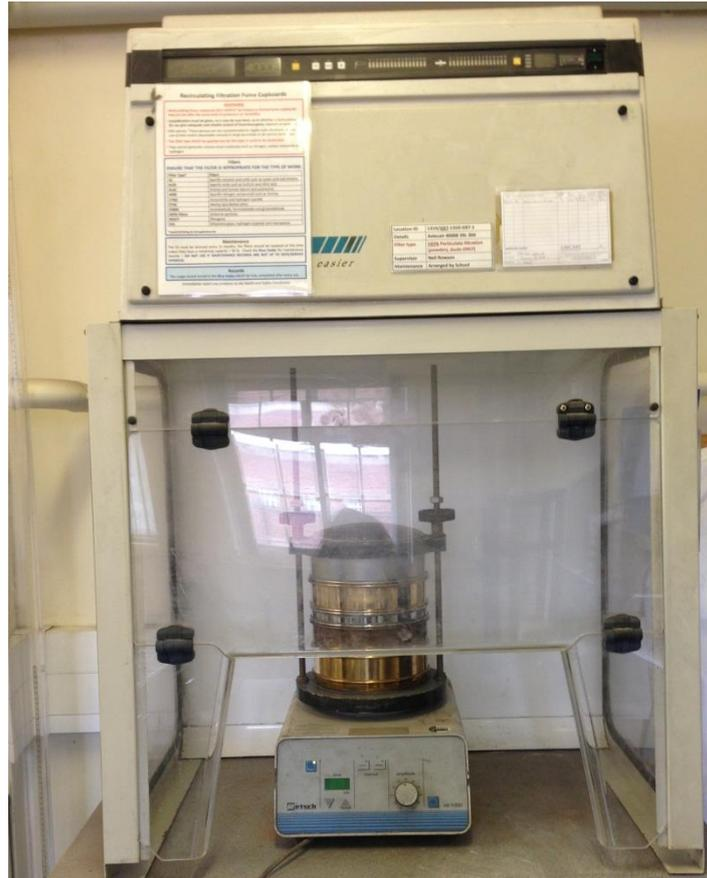
**Figure 4.2 - Agitated Dry Sieving Set-up**
