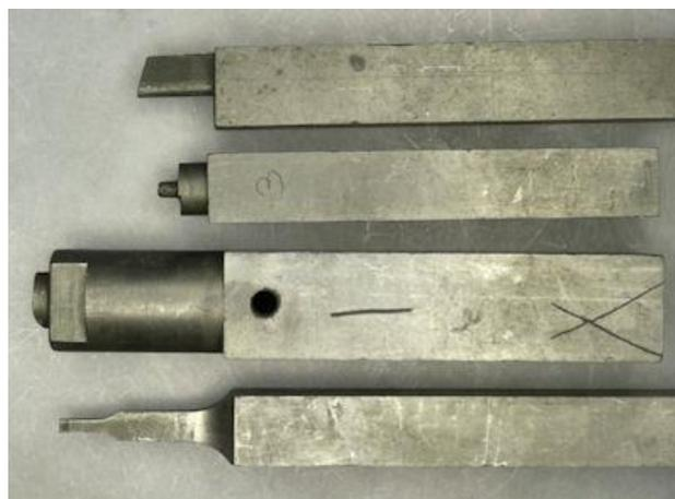
**Figure 1.13: A selection of graphite electrodes (robotroom)**
