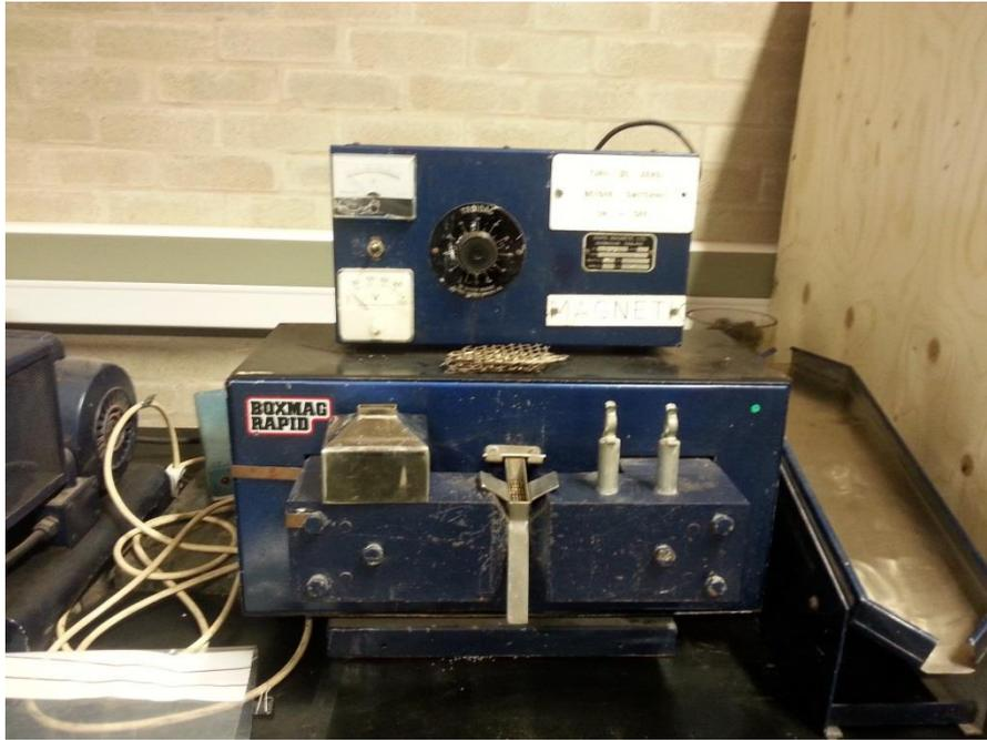
**Figure 4.4: The wet magnetic separator used**
