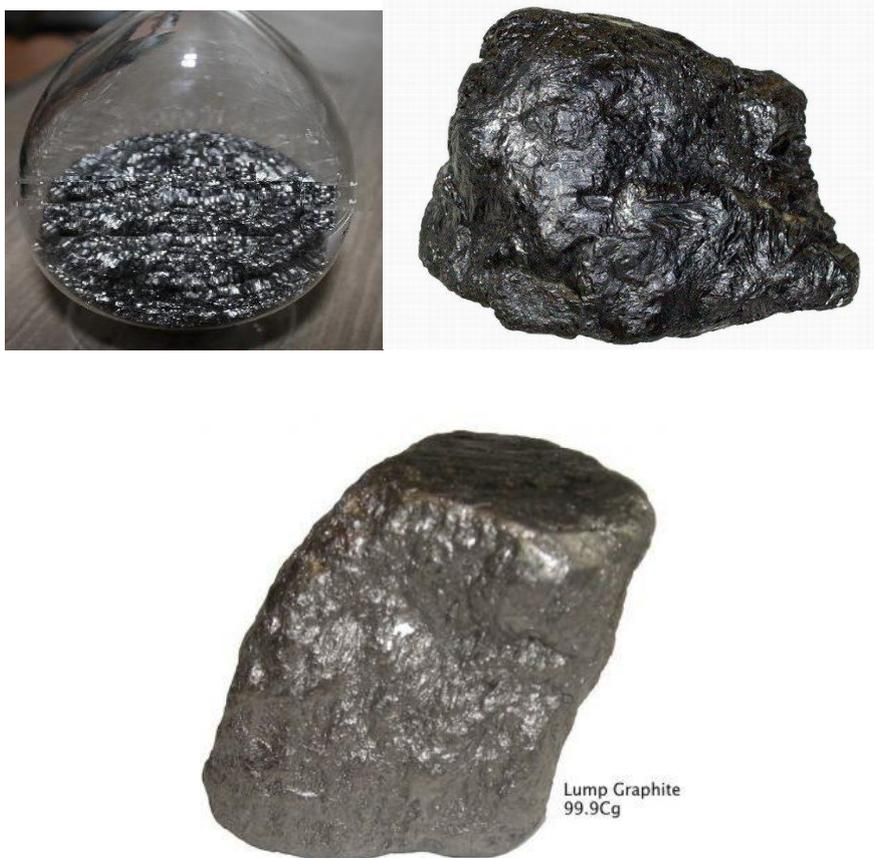
**Figures 1.6, 1.7 and 1.8 (clockwise from top left): Examples of flake, amorphous and lump (vein) graphite (made-in-china/grupolandfer/saintjeancarbon)**
