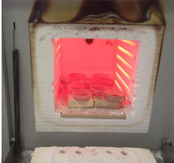
**Figure 4.8: LOI test furnace with door open to allow cooling of crucibles**
