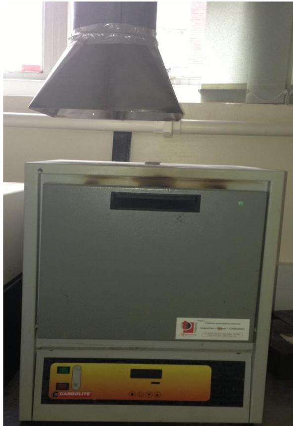
**Figure 4.7: Carbolite Burn-off Furnace with extractor hood**
