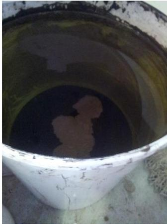
**Figure 4.3: An example of the kish slurry formed**
