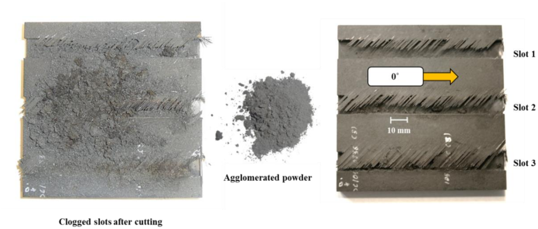
Figure 4.18: Burning of dust within slot Test-3
