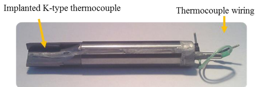
Figure 3.14: Implanted thermocouple in Exactaform router
