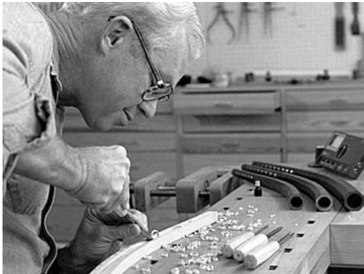
Figure 34: Cornett maker John McCann carving the internal bore of a curved cornett
