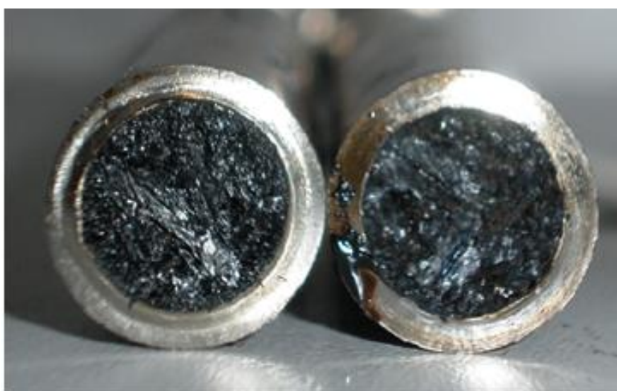
Figure 7.9 Photograph of coked Ni-Mo/Al 2 O 3 catalyst of the CAPRI reactor cross-section after upgrading at temperature 425 °C, nitrogen-to-oil ratio 500 mL.mL -1 , and pressure 20 barg (Reactor tube internal diameter 10 mm).
