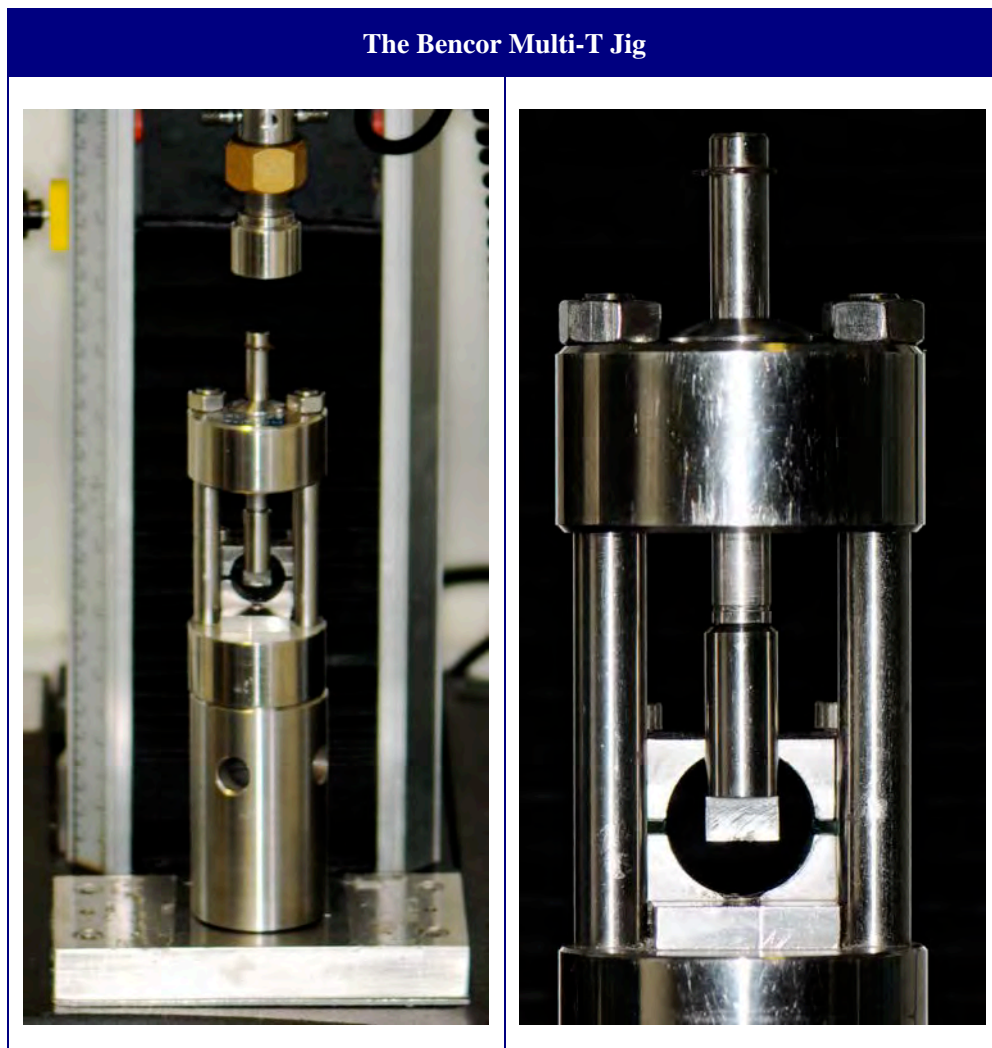
Figure 3.3 The Bencor Multi-T jig attached to the Instron testing machine
