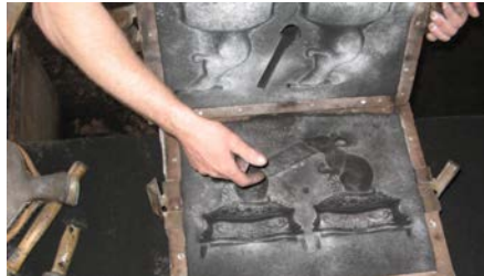
Figure 37 Casting a small ornament with green sand in a box at Blists Hill Museum (the author)
