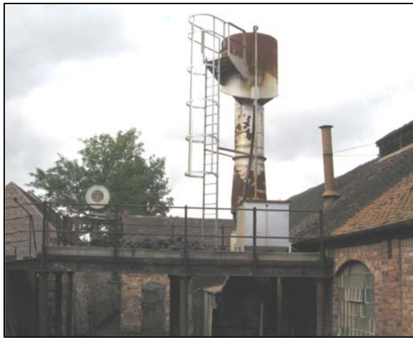
Figure 31 (above) – Cupola furnace at Blists Hill Museum (notice the external charging platform) (the author)
